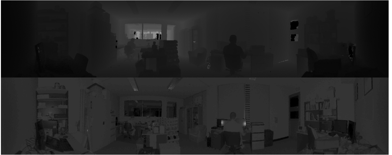
Figure 9: This image shows two identical 360^\circ \times 70^\circ cylindrical panoramas created using only four frames of the depth camera ( 90^\circ \times 70^\circ each). Top: panorama created using the depth channel. Bottom: panorama created using the 905 nm IR intensity channel.
