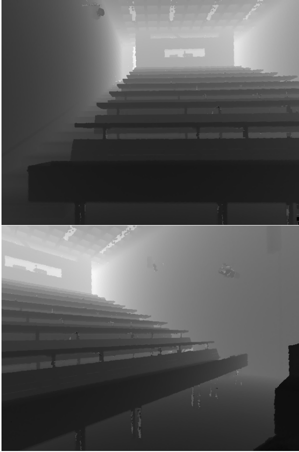
Figure 5: Top image shows a depth map of a lecture theatre (back wall 15 m away from camera) with a vertical field of view of 70^\circ projected on a 640 \times 480 image. The bottom depth map was captured by rotating the camera 45^\circ in azimuth. The user can set the configurable depth camera horizontal angle of view by changing the aspect ratio of the projected image. This allows the user to specify the exact region of interest in the scene for each frame.
