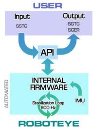
3-axis stabilization - Not only is stabilization about three axes rare in a form factor comparable to the REV25-ST, the REV25-ST delivers stabilized motion about yaw, pitch and roll<sup>1</sup> at the high levels of performance characteristic of RobotEye Vision systems.
