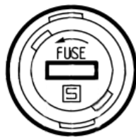
Figure 3.1 – Fuseholder on the RE05 Enclosure
